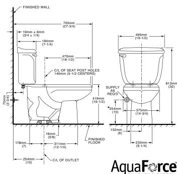
THIS TOILET IS DESIGNED TO ROUGH-IN AT A MINIMUM DIMENSION OF 254mm (10") FROM FINISHED WALL TO C/L OF OUTLET. SUPPLY NOT INCLUDED WITH FIXTURE AND MUST BE ORDERED SEPARATELY
